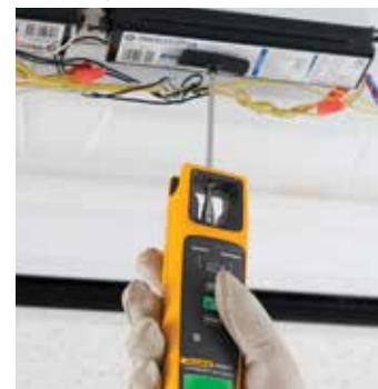
Easily determine if ballast is working.
