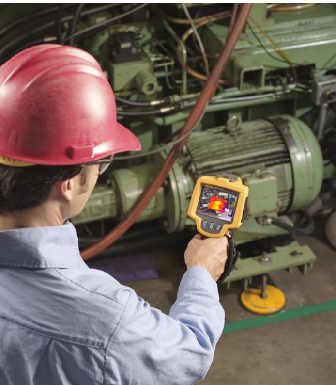
Figure 1. Thermal imagers offer a quick way to inspect equipment for abnormally hot-spots, and piping for abnormally cool spots.
