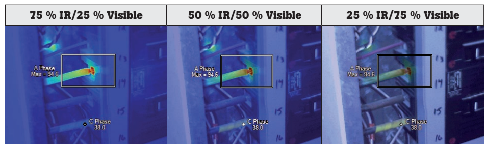
Figure 2. Percent IR/visible blending can be adjusted for optimum interpretation
