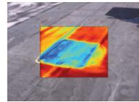
Figure 2: Wet insulation in flat roofs can cause rotting unless detected and corrected.
