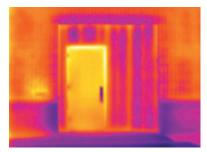
Figure 1: Energy loss via the door of a building.
