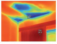
Figure 5: Thermal resolution for the TiR Series is as low as 0.07 ° Celsius. This gives the clearest possible view of possible problem areas.
