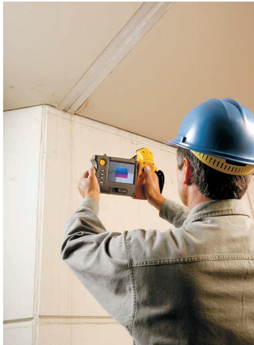
A diagnostic site visit can reveal the hidden dynamics and interactions between the building shell, heating system, and other building features. Here, a **Fluke TiR thermal imager** reveals missing insulation, which is a major contributor to heat loss.
