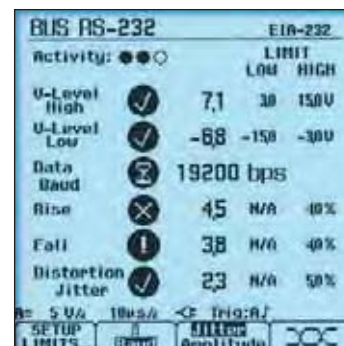
Bus Health mode allows for an analysis of the signal quality on an industrial network.
