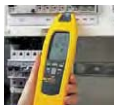
Location of fuses/breakers and assignment to circuits
