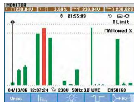
The System-Monitor overview gives instant insight into whether the voltage, harmonics, flicker, frequency and the number of dips and swells fall outside the set limits. A detailed list is given of all events falling outside the set limits.
