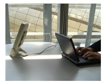
The Altai C1 an employs patented smart signal processing algorithms and antenna design to increase WiFi signal strength (transmit and receive) by as much as 18 dB in areas covered by an A8n Super WiFi Base Station or A2 WiFi Access Point. It can be installed exactly where the throughput is required to boost up, and it allows the service operator to increase the coverage range of an A8n base station substantially and provides greater flexibility and cost savings to WiFi deployments.
