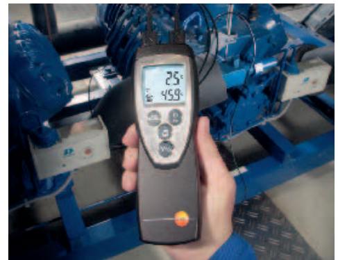
Simultaneous measurement of overheating and undercooling in refrigeration systems with testo 922
