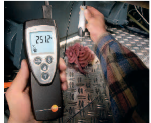
Temperature measurement in semi-solid materials with the superfast penetration probe, ideal for plastics, foodstuffs etc.
