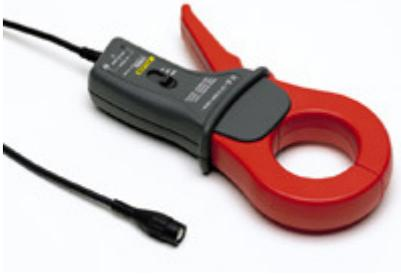
The Fluke i1000s is a clamp-on ac current probe designed to expand oscilloscope applications in industrial and power environments. The Current Probe (shown in figure) provides the following features: Ideal for measuring distorted current waveforms and harmonics.
