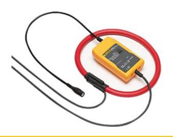
The i6000sflex is an AC current probe utilising the Rogowski principle. It can be used to measure currents up to 6000A when used in conjunction with oscilloscopes, recorders or data loggers. The flexible and lightweight measuring head allows quick and easy installation in hard to reach areas.
