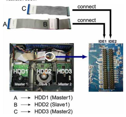
**NOTE:** If you plan to install external disk array, please don't install the HDD in the "HDD3" postion.
