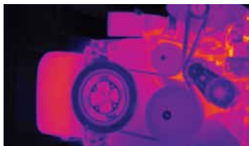
Inspection of the cooling system, exhaust system and transmission system for design improvement. 對發動機的散熱系統、排氣系統、傳動系統進行熱分佈檢測，改善設計
