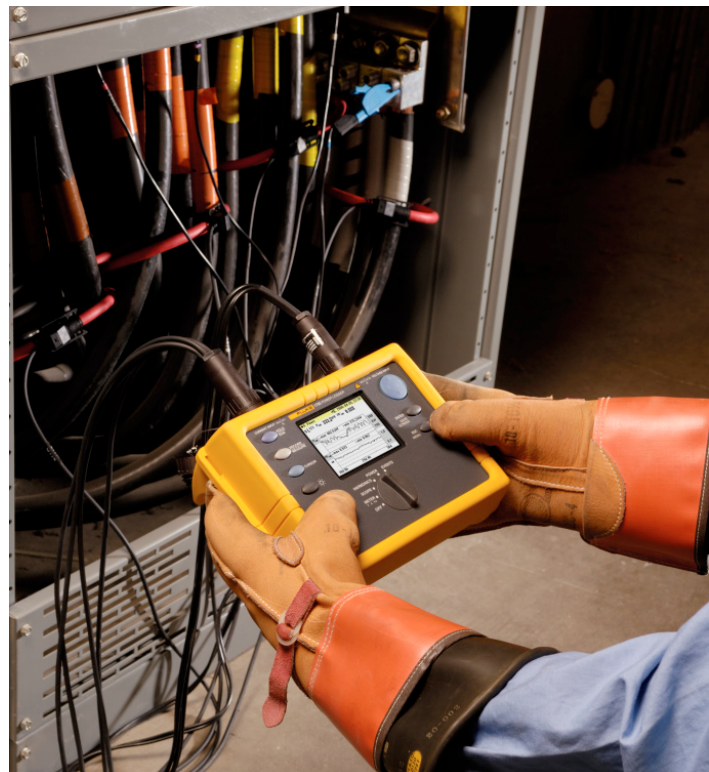
A three-phase power logger can measure demand over time, which can help identify areas where companies can cut energy costs.
